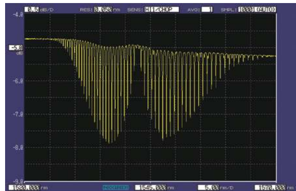
Hydrogen Cyanide \text{H}_{13}\text{C}_{14}\text{N} absorption spectrum measurement with AQ6375B
