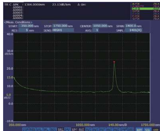
Measurement example of wavelength loss characterization with AQ6374
