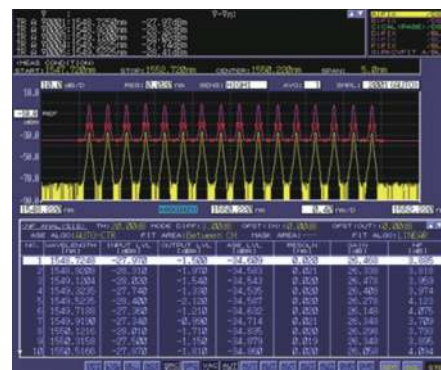
Figure 3 – The automated routine for the analysis of optical amplifiers provides a table with their relevant parameters
