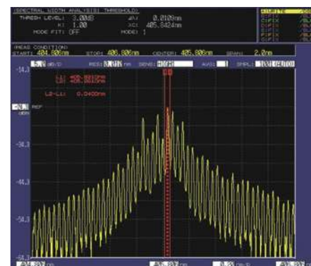
405 nm FP-LD measurement (resolution setting: 0.01 nm)
