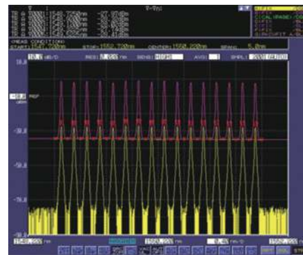
Figure 2 – Typical measurement result showing two traces; one before amplification (yellow) and one after amplification (purple).
